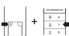
Simultaneously press on the control [Setting button] and [Stop] for 4 seconds
